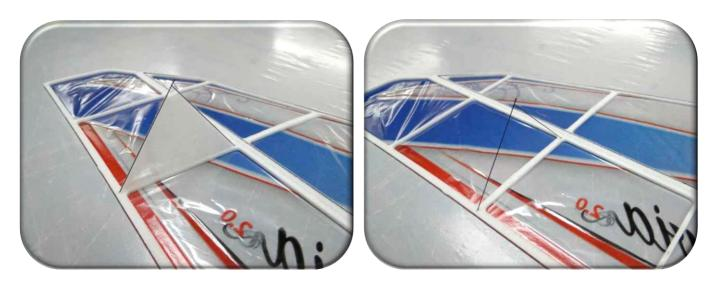
Take the Depron triangle template marked AIL position it on the aileron as shown and glue two 0.5rods.
