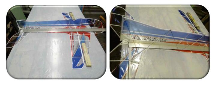
Go on with the main lower fuselage structure – 0,7mm carbon rods – number 6, 11 and 2, 4, 6, 7,
