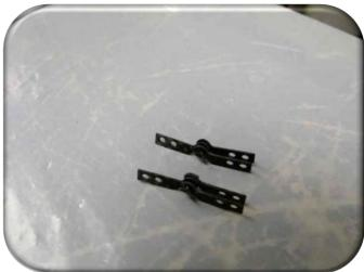
Prepare the carbon hinges. From a 1,5mm carbon rod cut 3 pieces of 8mm in length. Best way is to cut them at 15mm and then sand to the correct length.
