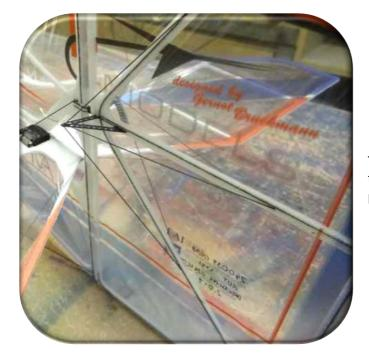
To get the rudder linkage even more precise, we recommend to strengthen it with 6x 0,5mm carbon rods as shown in the picture left.
