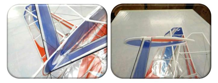
To make the landing gear strong enough you have to reinforce it with 0,5mm carbon rods – see the picture above. The last step is to mount the wheel pants. Cut the edge of the landing gear covers to 45° to get a perfect fit with the wheel pants.
