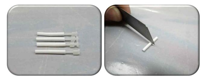
Cut the plastic tubes (are included with the Glavak motor) to the length of 12mm – don't cut away the end of the tube with the thread for motor screws.
