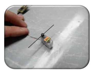
Then insert a 1,0mm carbon tube into the servo's output shaft hole.
