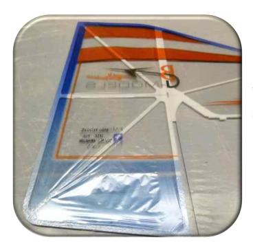
Next step is to hinge the rudder to the fuselage. The best way for this is to use UHU Por. Add a thin layer of glue to both sides and wait a few minutes, then put both parts to a flat table and move them together.
