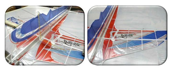
Start with the wing reinforcement – 0,7mm carbon rod – number 6 and 7
