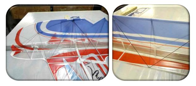
Next step is the nose section with 0.5 carbon rods – number 8, 5, 4, 2, 1
