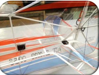
Glue the rudder servo to its slot and reinforce it with 2x 0,5 carbon rods.
