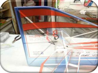
The rudder and the upper fuselage must be absolutely VERTICAL – so take your time and do it perfectly. Bet way is to glue the carbon rods fist to the horizontal fuselage so the upper part can be still adjusted before gluing.
