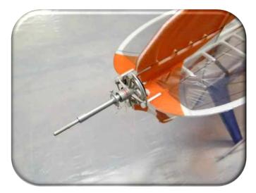
Screw the motor to its mounting tubes. Make sure to put the silicon separators between the tubes and the motor's mounting cross. Set to motor to 0 down and side thrust as good as possible – the final adjustment will be made in the first test flights.
