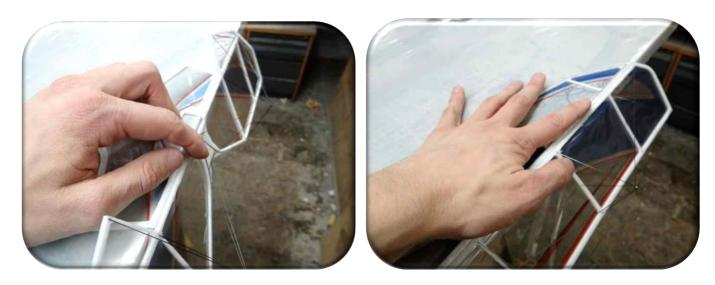
Position the aileron and elevator to the end of the table and bend it up and down a few times. To make sure that it can move easy.
