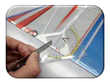
With a sharp knife split the fuselage in half
