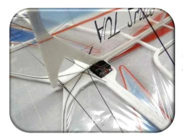
If the elevator servo is centered, glue it to its place. Attention: the servo's pivot should be at the same height as the hinge line.
