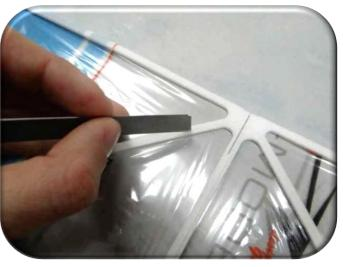
In the sketches you can find the right length and all positions for the 1,5x0,13mm carbon profiles. For gluing the profiles use really thin CA, pay attention to the amount of glue you use. Place the airframe parts on a flat working surface and weight them down, this will prevent bending of the parts as you insert and glue the profile reinforcements.
