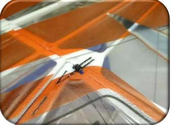
Check if the hinges and the rudder control horn fit the slots. If yes glue them with CA – be careful the surfaces should still move easily.
