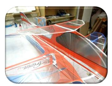
When the upper part is fully reinforced, glue the top canaliser to the fuselage and reinforce it.
