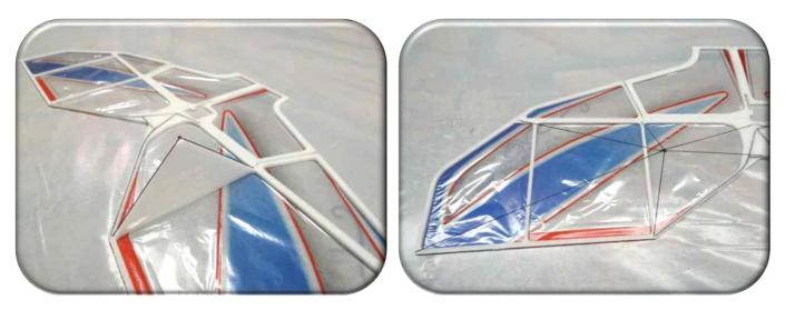
Take the Depron triangle marked ELE and glue the 2 0,5mm rods. Make sure that everything is straight and arrange the carbon rods as shown in the 3D sketch and glue them to the triangle and Depron.
