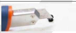
Insert the CHC M5-45 screw and the first spacer. Insert the wheel inside, place the second spacer, and lock the set by mean of a M5 nut-locking.
