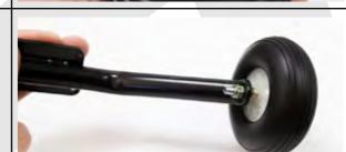
For the front gear preparation, shorten with a cutter the two spacers, from 1 to 2 mm.
