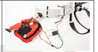
Install the ballast into your pilot, in fact of the harness (modulate the ballast quantity according to the wing size and the weather conditions of the day).
