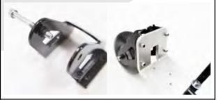
Remove the fixation beads of the speed controller. Arrange then the rear landing gear and fix it by mean of 4x CHC M4-12 screws and M4 nutlockings. The speed controller can be fixed again on the rear landing gear.
