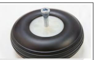
Lock the screw by mean of a M5 nut-locking. Do not completely tighten it, in order to let the wheel rotate
