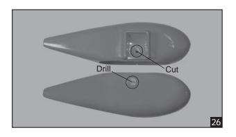
3. Using a modeling knife, carefully cut out two line from the margin of the hole onto the wheel pant.
