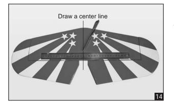
Check the fit of the horizontal stabilizer in its slot. Make sure the horizontal stabilizer is square and centered to the fuselage by taking measurements, but don't glue anything yet.
