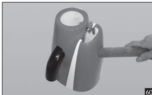
3. Slide the cowl back into place. Align the front of the cowl with the crankshaft of the engine. The front of the cowl should be positioned so the crankshaft is in the middle of the precut opening. Hold the cowl firmly in place using several pieces of masking tape.
