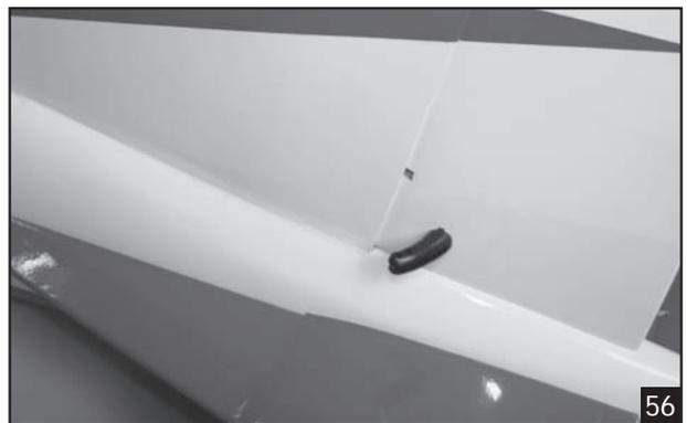
3. Working from inside the fuselage, slide the threaded end of the remaining pushrod down the inside of the fuselage until the pushrod reaches the exit slot. Carefully reach in with a small screw driver and guide the pushrod out of the exit slot.
