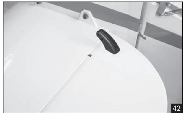
**INSTALLING THE ELEVATOR PUSHROD**
