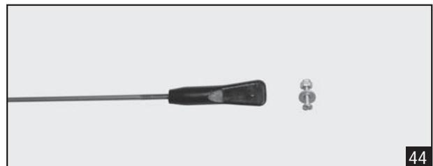
4. Install the nylon clevis into the two elevator pushrod. Make sure 6mm of thread shows inside the clevis.
