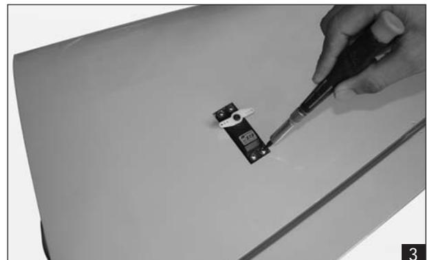
5. Repeat step # 2 - # 4 to install the second aileron servo in the opposite wing half.
