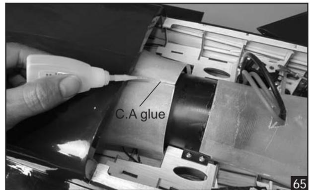
6. Glue the wooden belt for EDF (Included with the kit) using C.A glue.
