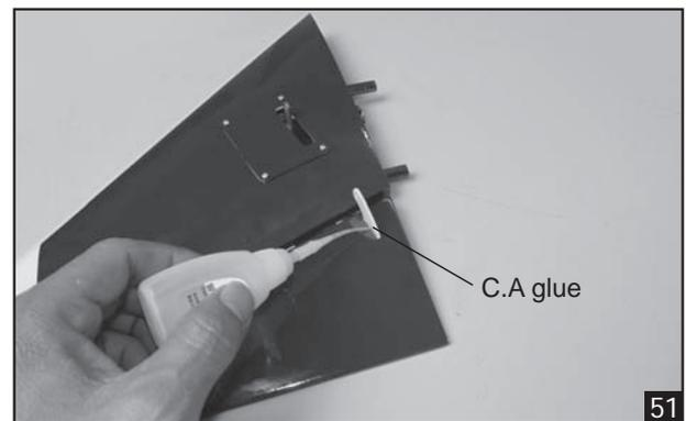
7. Repeat these step from installing the aileron linkages to install the rudder linkages.
