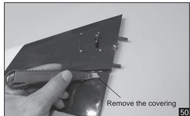
6. Install and glue the rudder control horn.
