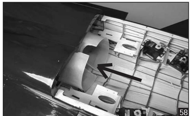
2. Slide the air outlet to the fuselage.
