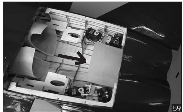
3. Trim 1 hole from the air outlet for the wires of EDF.
