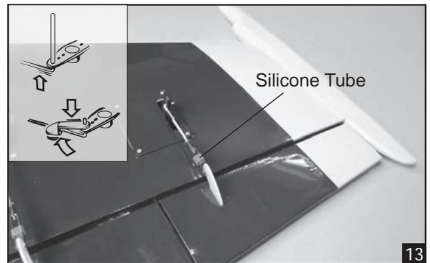
8. Insert the 90 degree bend down through the hole in the servo arm. Install one nylon snap keeper over the wire to secure it to the arm. Install the servo arm retaining screw and remove the masking tape from the aileron.
