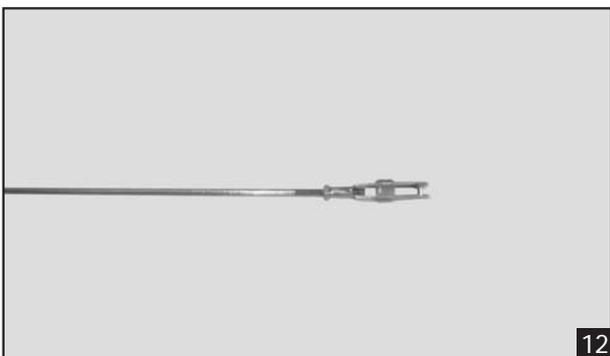
2. Attach the clevis to the outer hole in the control horn. Install a silicone tube on the clevis.
