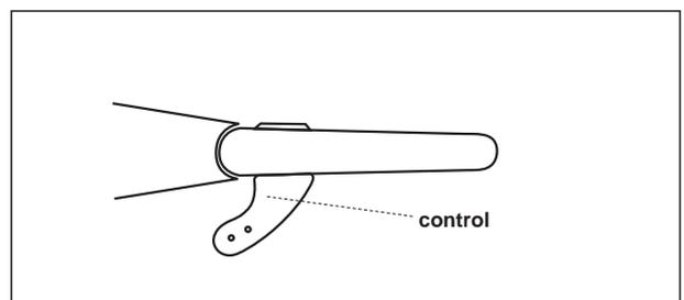
**INSTALLING THE CONTROL HORNS FOR FLAP**
