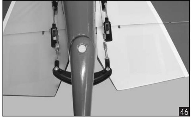
6. Center the rudder servo using the radio and install the servo arm. Attach the metal clevis to the rudder servo arm.
