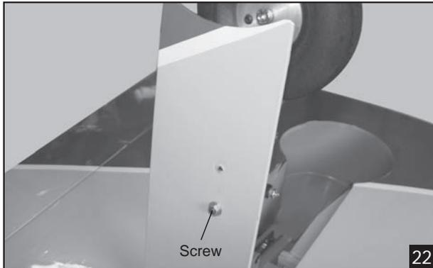
11. Secure the wing to the fuselage using the plastic screws.
