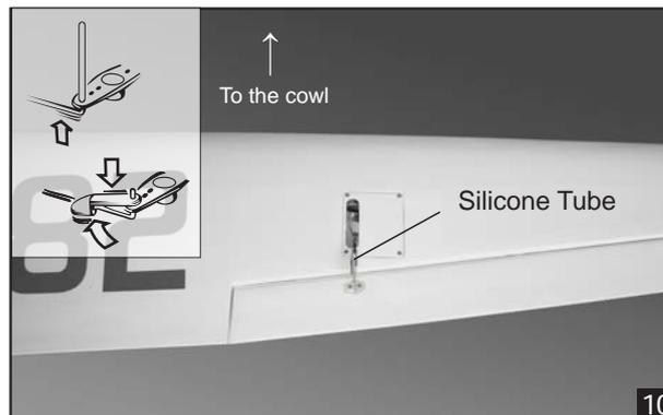
9. Repeat step # 4 - # 8 to install the second aileron linkage. After both linkages are completed, connect both of the aileron servo leads using a Y-harness you have purchased separately.
