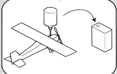
Empty the fuel tank after flying, fuel left in the tank can cause corrosion and lead to engine problems.
