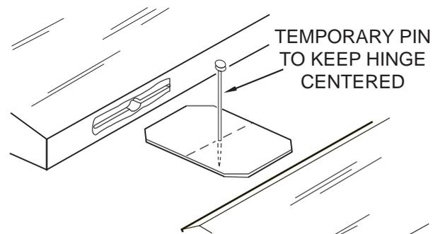
5. Apply six drops of thin CA to the top and bottom of each hinge. Do not use CA accelerator. After the CA has fully hardened, test the hinges by pulling on the aileron.
