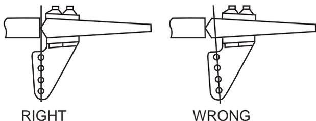
3. Repeat step # 1 - # 2 to install the control horn on the opposite aileron.
