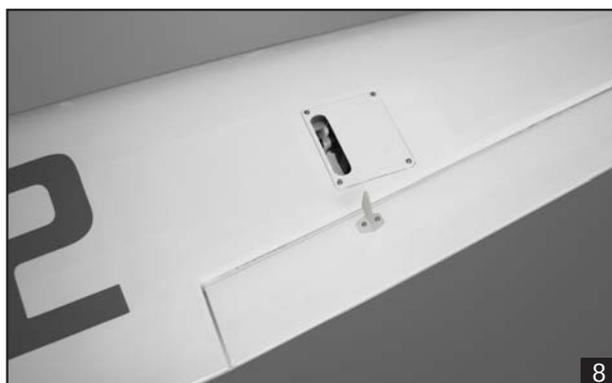
6. With the aileron and aileron servo centered, carefully place a mark on the aileron pushrod wire where it crosses the hole in the servo arm.
