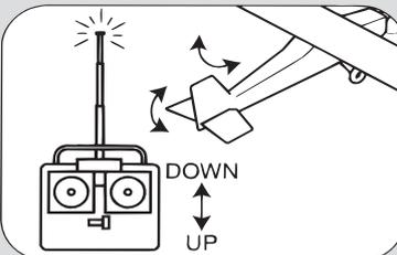
Operate the control sticks on the transmitter and check that the control surfaces move freely and in the CORRECT directions.
