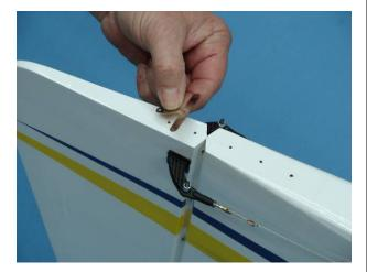
3. Apply a drop of thick CA to the tiller arm mounting screws before inserting in the predrilled holes.
