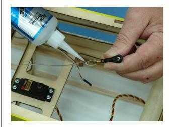
31. Attach ball links to the rudder servo arm and then attach the servo arm to the rudder servo as shown.
