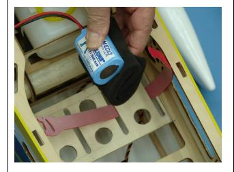
5. Install battery using foam padding and securely tighten one wrap strap as shown.
