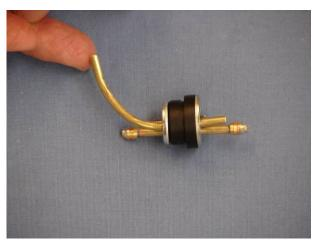
7. Install the fuel tubing and clunk. Secure the fuel tubing with nylon ties to the pick-up tube and clunk.
