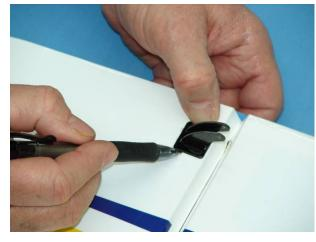
7. Use a hobby knife to carefully remove the covering. Take care not to cut too deep and damage the wood underneath the covering.
