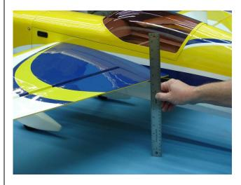
2. Use the widest part of the elevator as shown to measure the elevator throw in inches.
