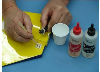
15. With elevator centered in natural position, ensure the mounting hole of the control horn is centered on the hinge line as shown. Double check this alignment while the epoxy cures, it is very important that the control horn is correctly aligned with the hinge line.
