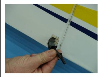
13. Apply 30 minute epoxy to the remaining base plate and install on the rudder control horn. Ensure both base plates are fully seated against the rudder before the glue fully cures.
