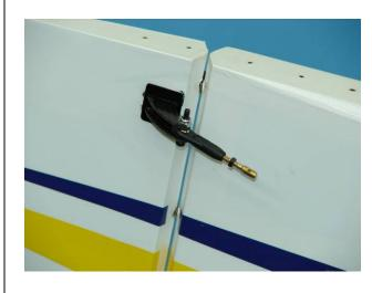
19. Finished 4-40 coupler installation, ensure that both sides are of equal length for easy adjustment and proper deflection.
