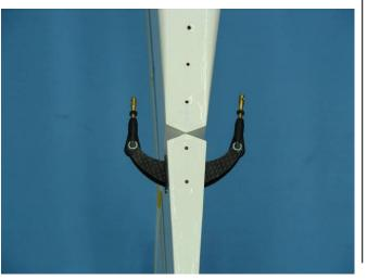
20. Install the rudder servo in the servo cutout with the output shaft to the nose of the airplane.
