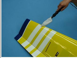
6. Go over all hinge gaps to ensure there are no wrinkles. Excessive wrinkles in the hinge line can cause binding and or damage to the covering.
