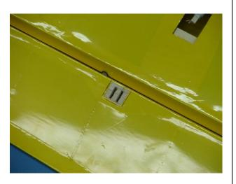
7. Apply 5 minute epoxy into the control horn mounting slots and the base plate mounting location as shown.
