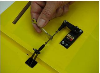
19. Final aileron servo installation shown below, repeat all previous steps for the remaining wing assembly.
