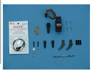
2. Use 80 Grit Sandpaper to scuff the carbon control horn and base plate where it will be glued to the aileron as shown below.
