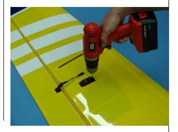
15. Install servo with servo mounting screws. Repeat servo installation process for remaining aileron servo.
