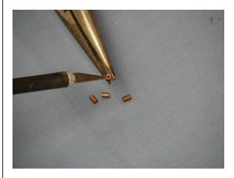
25. Thread cable through brass swage tube.
