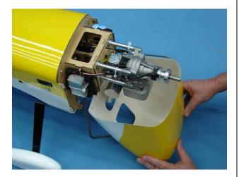
20. Bolt cowling in place and check the stinger exit location at this time. If the cowling comes into contact with the exhaust at any point, remove cowling and enlarge the stinger cutout for a proper fit.
