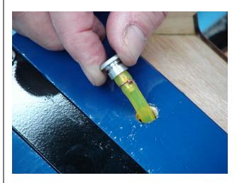
17. Use thick CA to secure fuel vent exit dot in fuse.
