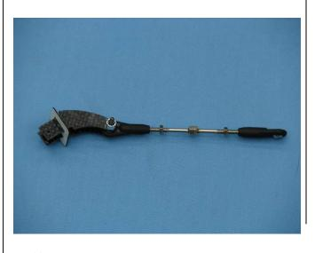
11. Place elevator control horns into the pre-cut slot with the base plate installed. Use a ballpoint pen to mark the location of the base plate as shown below.
