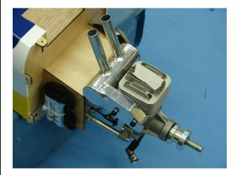
13. Reinstall the cowl template and mark the location of the muffler exit stingers at this time.
