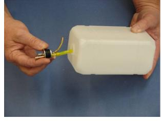
9. Secure the rubber stopper with set screw. Take care not to strip threads by over tightening set screw.
