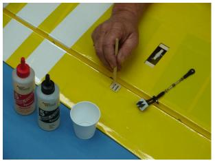
8. Place aileron control horn into the pre-cut slot. Wipe away any excess epoxy that may have come out at this time. Ensure that the base plate is making full contact with the aileron at this
