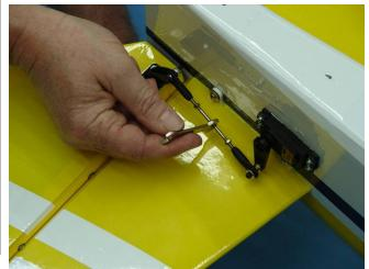
19. Final elevator servo installation shown below. Repeat all previous steps for the remaining elevator assembly.
