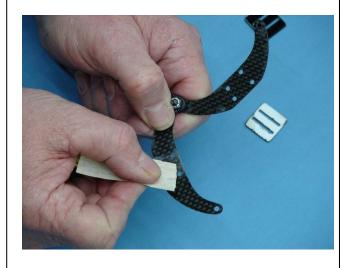
9. Use 80 grit sandpaper to lightly scuff the back of the control horn mounting base as shown.
