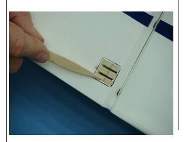
12. Slide the upper and lower rudder control horn into the pre-cut slots as shown. Ensure that the control horn is centered on both sides before the epoxy fully cures.
