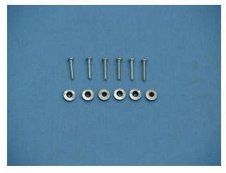
2. Mount the cowl using the cowl mounting bolts and rubber backed washers. The rubber backed washers are to prevent the fiberglass cowl from cracking and to prevent mounting bolts from loosening from normal engine vibration.
