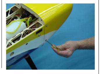
3. Gather (2) 6-32 wing mounting bolts, (2) #6 rubber backed washers and (4) hairpins for preparation of mounting the wings.
