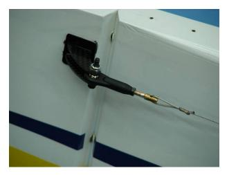
35. Finished ball link pull pull installation shown below.
