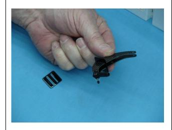
3. Slide upper and lower rudder horns through the pre-cut slot in the rudder as shown below.
