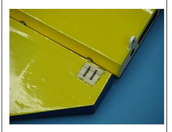
14. Apply 5 minute epoxy into the control horn mounting slots and the base plate mounting location as shown.
