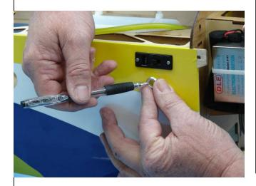
10. Use a hobby knife to remove covering followed by the underlying balsa as shown below. The use of a new blade is recommended for a clean, easy cut.
