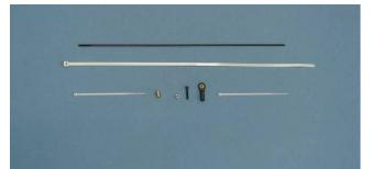
2. We recommend installing the carburetor choke pushrod as shown. Use nylon ties to provide support and holding friction for the choke pushrod. Place silicon fuel tubing over the wire pushrod to prevent damage from vibration and provide holding friction. Solder a threaded insert on the end of the pushrod to provide a finger grip.
