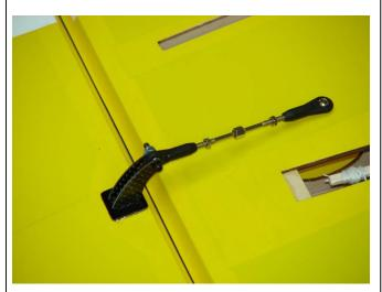
9. With aileron centered in natural position, ensure the mounting hole of the control horn is centered on the hinge line as shown. Double check this alignment while the epoxy cures, it is very important that the control horn is correctly aligned with the hinge line.
