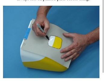
10. Remove the template and use a rotary cutting tool and sanding drum to cut out the openings in the cowl.
