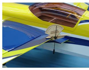
9. Use the widest part of the elevator to measure the elevator throw in degrees.
