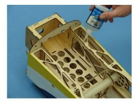
2. Use thin CA on the front canopy mounting tabs as shown. **<u>DO NOT</u>** install canopy on the fuse until glue has fully cured. Failure to do so may cause canopy to be permanently glued to the fuse.
