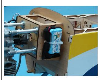
6. The ignition switch mounting location is at builders discretion. Mark the location for the ignition switch using the switch mounting plate for a template. Use a modeling knife to cut out the switch hole.
