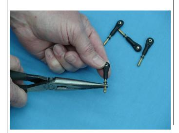
18. 4-40 coupler shown attached to the rudder control horn ball link.
