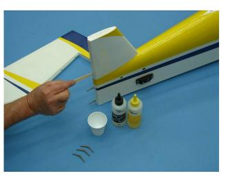
4. Epoxy the hinges into the fin first and allow epoxy to fully cure.
