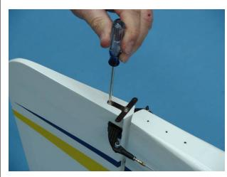
5. Align the tail wheel with pre drilled mounting holes on the bottom of the fuse.
