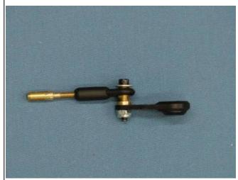
9. With servo arm still 90 degrees to servo and throttle arm of carburetor in the center or half throttle position. Mark the cut location for the throttle push rod.
