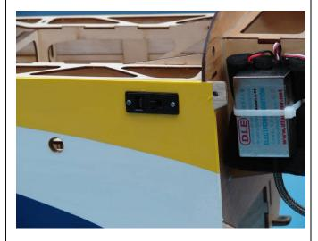
8. Mount ignition regulator as desired. Secure all connectors with tape, safety clip or similar.
