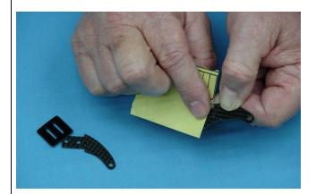
3. Assemble the pushrod and control horn assembly as shown. The ball link goes between the left and right sides of the control horn sides and is secured with a nylon lock nut. Brass spacer goes between servo arm and ball link and is not installed between the right and left control horns
