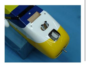
21. Locate the supplied front air inlet template and tape to cowl using masking tape.
