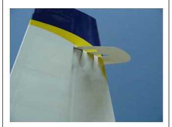
6. Degrees are measured at the tip of the boost tab as shown below.
