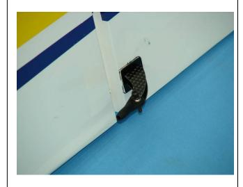
15. Before the epoxy has fully cured ensure that full rudder travel can be achieved. If the control horns come in contact with the fuse at full throw they may not be properly centered in the slots.
