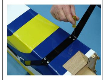
5. Install the axle into the gear strut with lock nut. Lightly tighten axle lock nut at this time.
