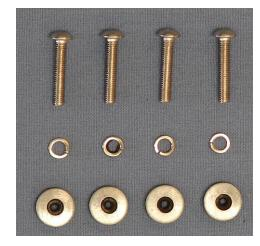
8. Slide the stab tube in the fuse stab tube sleeve. Slide the stabs on the stab tube and connect pushrod to servo arm. Slide the rubber backed washers on the stab mounting bolts and insert bolts through the stab mounting tabs and into the fuse blind nuts. Tighten snugly but do not over tighten and crack the stab mounting tabs or the fuse sides.
