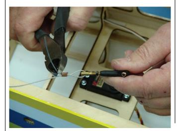
34. Attach the ball link to the rudder control horn as shown below. Follow the same steps as shown in the previous pages to install the ball link to the pull pull cable.
