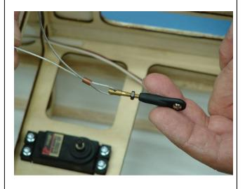
27. Loop the cable back through the brass swage tube and pull tight.
