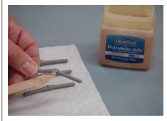
3. Mix epoxy in mixing cup and use a tapered stick to apply the epoxy inside the pre-drilled holes in the trailing edge of the fin. Apply epoxy to one side of each hinge and insert the hinge completely into the hole. Ensure the hinge axis is vertical and parallel to the trailing edge of the fin before epoxy cures. Wipe away excess epoxy with alcohol wetted wipes.
