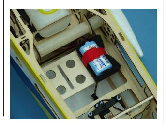
6. Attach hook and loop material to the backside of the regulator as shown.
