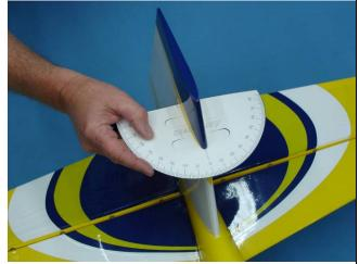
5. Secure the tabs to the fin using clear tape.
