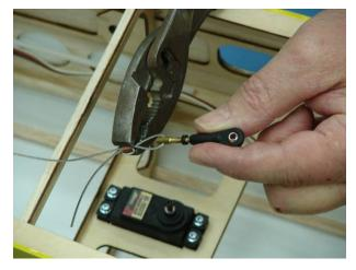
29. Cut off excess cable as shown.
