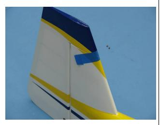
33. Plug the rudder servo into the rudder channel of the receiver and power up. Turn on transmitter to center rudder servo. Ensure servo trim and sub-trims are centered.
