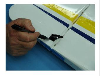
5. Slide the remaining base plate onto the opposite side of the rudder control horn as shown.
