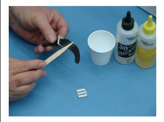
11. Apply 30 minute epoxy to the rudder as shown. This will only be done on the side of the rudder that has the corresponding base plate already installed on the control horn.
