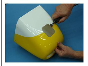
11. Temporarily mount cowl to fuse, ensure that the cowl does not come in contact with the engine and that there is at least 1/4" of clearance between the cowl and the motor. Make any adjustment to the cylinder head cut out at this time.
