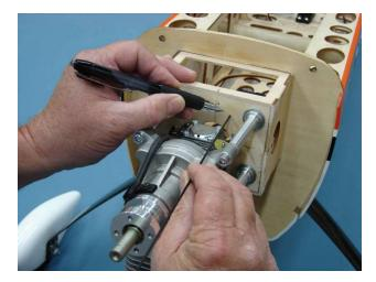
3. Use a drill bit to drill the holes for the throttle pushrod.
