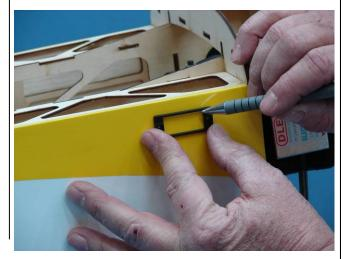
7. Mount switch in accordance with the switch manufacturers instructions and hardware.
