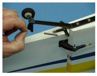
9. Wrap spring around steering tiller and then back around itself as show below. This is best performed by hand but pliers can also be used.
