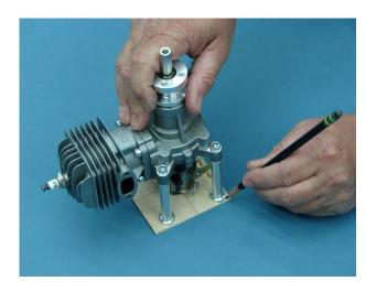
5. Use a stencil to fill in any missed parts where the standoffs were marked in step 4.
