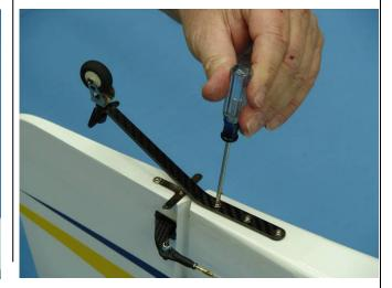
8. Attach the steering spring to the rudder tiller. Center the spring between both tail wheel and steering tillers.
