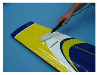
3. If bubbles persist, use a small pin to punch holes in the bubble to relieve trapped air and reheat.
