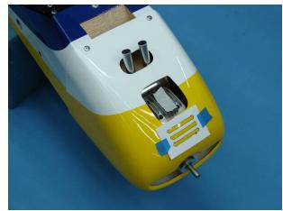
22. The front air inlets should be centered both vertically and horizontally on the engine head. This will allow cool air to pass through the cowl and into the fins of the engine.
