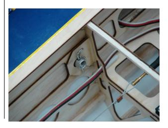
7. Gather (4) 4-40 stab mounting bolts and (4) #6 small rubber backed washers, these will be used to secure the stabs to the fuse.
