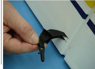
4. Place base plate against rudder and mark its location with a ballpoint pen.
