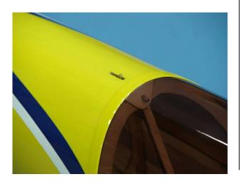
11. Ensure that the front hold down dowels, center hooks and canopy latch are all engaged. If the hold down dowels or center hook is not fully seated the canopy latch will not lock into the canopy.
