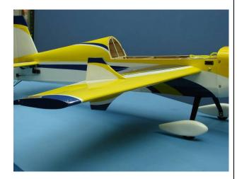
8. Mount the outer SFG using the supplied 4-40 mounting bolts and #6 bonded washers.
