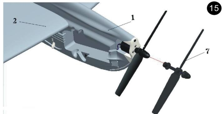
Install propeller collet and its base on motor. Please check if propeller is fixed well before flying.
