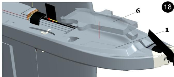
Cover the equipment cabin canopy. To avoid missing equipments while flying, please check if magnets on canopy and fuselage are stucked firmly before flying.
