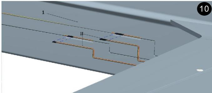
Connect elevator & rudder servo extension to servos and embed them into the slots on fuselage, refer to above picture. Make sure the colors of servo wire are correct while assembly.
