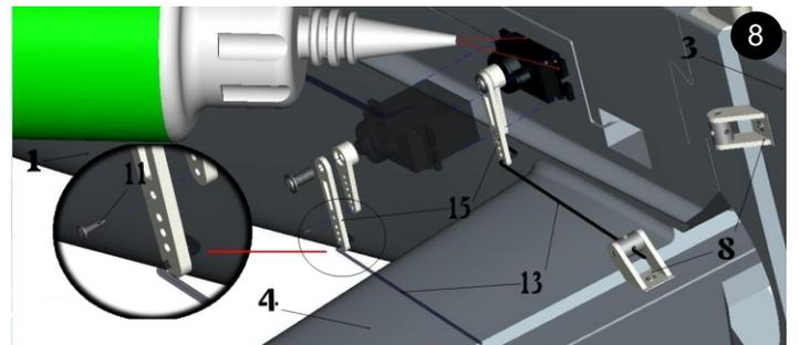
Install elevator servo on fuselage and fix with glue. And install the servo arm extension as picture shown. Then embed servo wire into the slot on fuselage.
