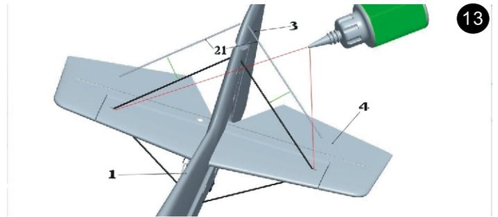
Install upper stabilizer bracing rods onto the slots of stabilizer and rear fuselage, then fix with glue. Make sure stabilizer is perpendicular to fuselage and rudder is on the same level as fuselage, no distortion.
