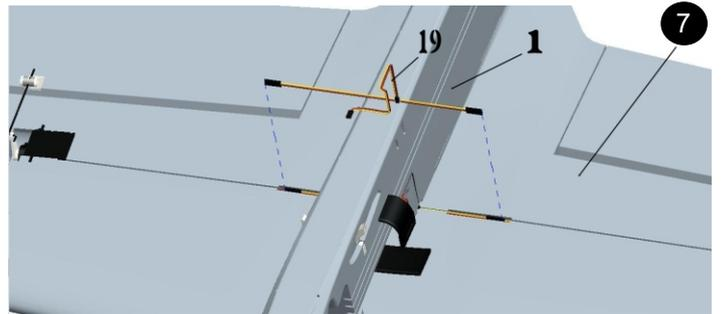
Use Y connector to connect left and right aileron servos. And embed the wires of Y connector along the slots on wing.
