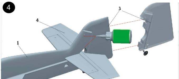
Attach rudder onto the rear fuselage according to their corresponding cuttings and fix with glue. Make sure the rudder is on the same level as fuselage.
