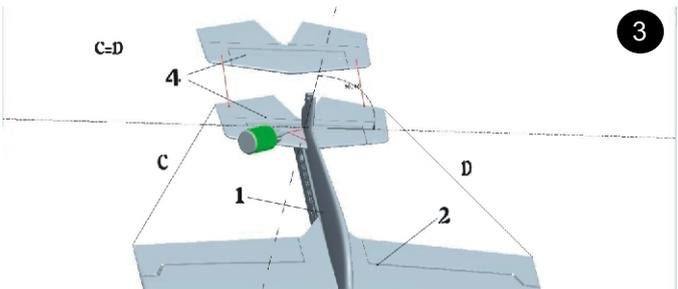
Insert stabilizer into the slot of rear fuselage and fix with glue. Make sure the fuselage is perpendicular to stabilizer and the stabilizer is centered, no excursion
