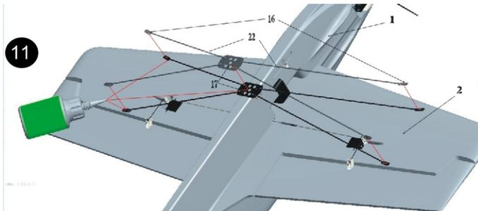
Install wing bracing rods with 1mm carbon fiber reinforcements and fix with glue. Please take notice on the installed places and directions of reinforcements while assembly.
