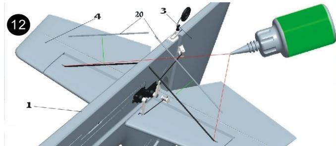
Install lower stabilizer bracing rods as picture shown. Make sure stabilizer is perpendicular to fuselage.
