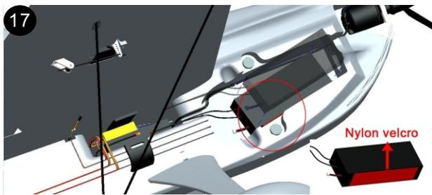
Place battery inside the slot of fuselage and fix with nylon velcro band. Please double check if battery is fixed firmly before flying. Then turn on transmitter and power on to do equipment test.
