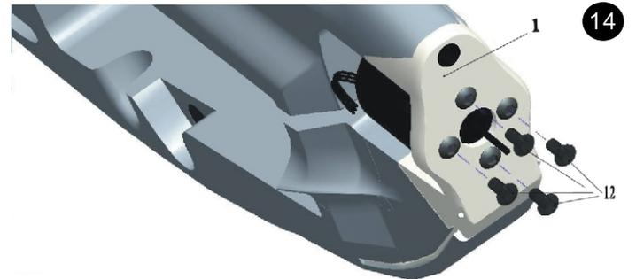
Install the motor onto the motor mount and fix with screws.
