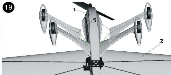
Separately insert left and right landing gear sets into the hub on fuselage, then drop some glue on the joints to fix.
