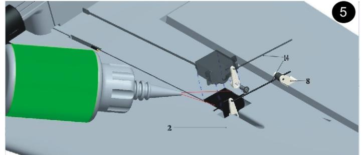
Use glue to fix servo into pre-cut place on wing, then connect servo and aileron control horn with connecting rod. Make sure the aileron surface is in neutral.
