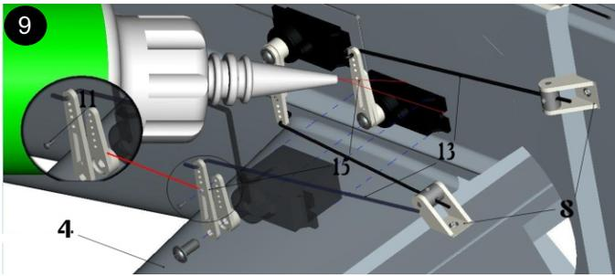
Install rudder servo, same step as elevator servo.
