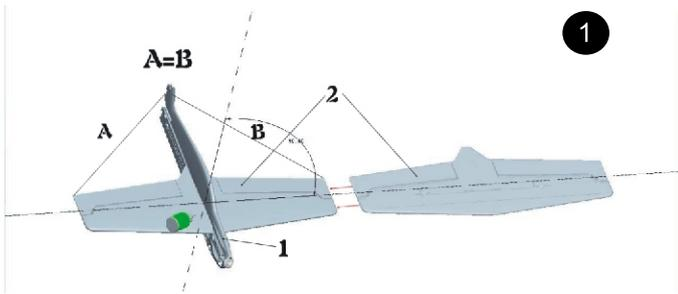
Insert wing into corresponding slots on fuselage, then use glue to fix. Make sure the wing without installed control horn pass through fuselage first, and ensure the wing is perpendicular to fuselage.
