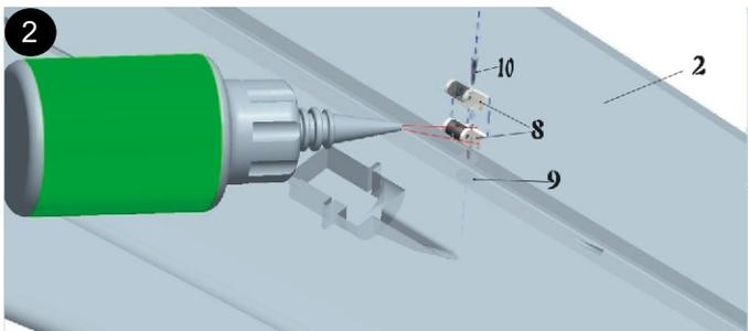
Install the control horns on another half of wing and fix with glue.
