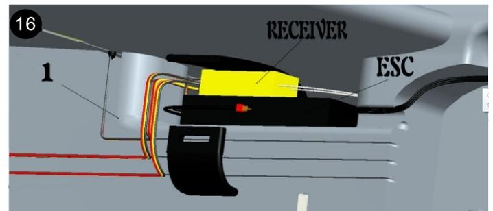
Place ESC and receiver into equipment cabin, and settle the wires as picture shown.
