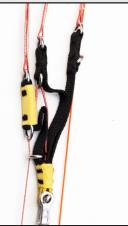
In accelerated position, the A must be lowered by 2cm maximum in order to guarantee a consequent speed gain and an optimal stability.
