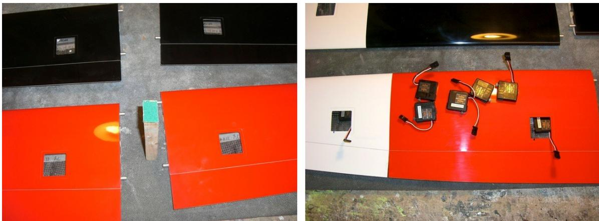
CA a piece of 80 grit sandpaper to a block as shown as use it to sand the inside of the servo bays lightly to prepare them for glue.
