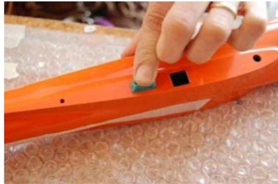
Then, through the wing joiner hole, put some thickened epoxy onto the back of the connectors to secure them really well.
