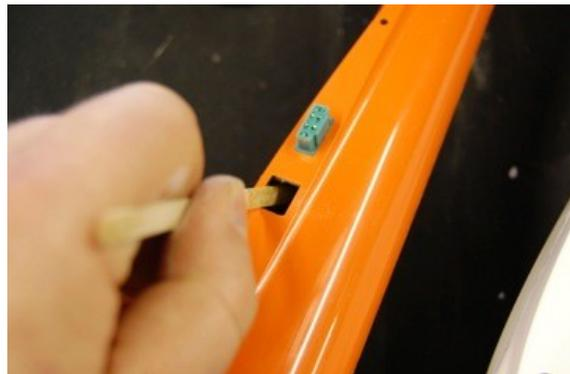
Securing the wing-side can be done as an automating connection, but the simplest way to do it is to simply leave the wing side loose and plug it on manually when sliding the wing on.
