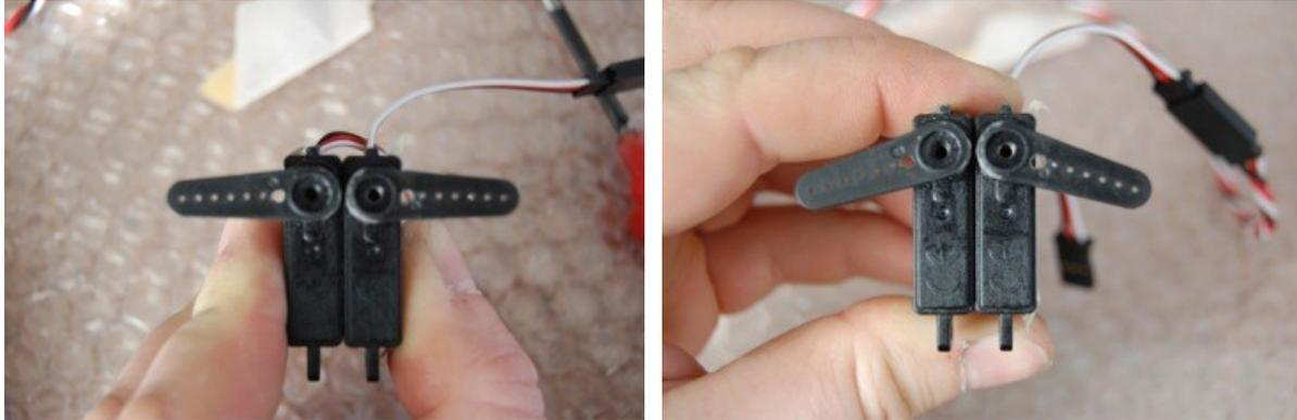
Once you have the holes in the arms, centre up your servos as shown. Ideally, do this with a servo tester. Note the subtrim numbers for each servo. Doing it with the arms untrimmed and left long makes it easy to get them symmetrically placed by eye.
