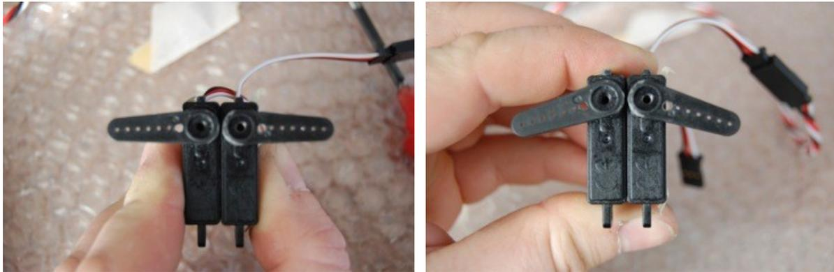
Once you have the holes in the arms, centre up your servos as shown. Ideally, do this with a servo tester. Note the subtrim numbers for each servo. Doing it with the arms untrimmed and left long makes it easy to get them symmetrically placed by eye.
