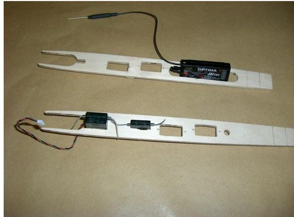
Note the marks at the rear of the tray. They show the position of the wing joiner. The tray runs underneath the wing joiner with enough clearance for the snakes to also go under the joiner. It is wise to put your fuselage wiring loom in place prior to gluing the tray in as this saves having to try to thread it through after the tray is in position!
