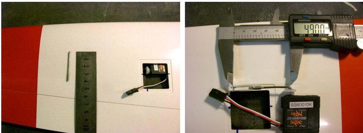
Cut the supplied pushrod to the length shown. Heat it up with a lighter or similar in a vice and slowly bend the threaded end as shown so that the length of the portion which goes through the servo arm is 7mm including the thickness of the pushrod. This is so that it will clear the servo casing when the servo is at full rotation.
