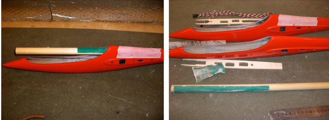
Glue some 80 grit sand paper to some 19mm dowel. If you don't have any dowel to hand, then you can just wrap some 80 grit paper around the actual ballast tube and secure it at one end with a wrap of masking tape. Use this to lightly sand the inside of the fuselage for the length of the ballast tube. Also, use some loose 80 grit sand paper to prepare the inside of the canopy area for gluing in the servo tray.
