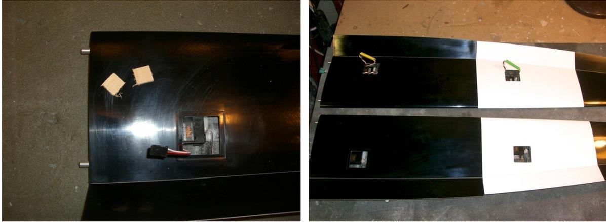
Then install the servo to the wing as shown. Ensure that the wiring loom is loose installed to the servos prior to gluing. Route the loom in FRONT of the servos to ensure that it does not interfere with the linkage. Put some heatshrink over the connectors to ensure that they remain secure. Bring the green mpx connector out through the hole provided in the wing root.
