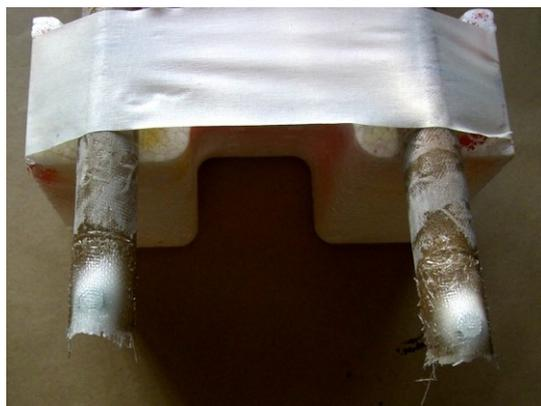
Mix up some epoxy and thickener and splooge around the nut from the underside. Cap it off with a layer of 100g glass cloth if you have some as shown. When dry, the bolt will easily unscrew due to the grease/ wax you put on the threads. That's your tube prepared!
