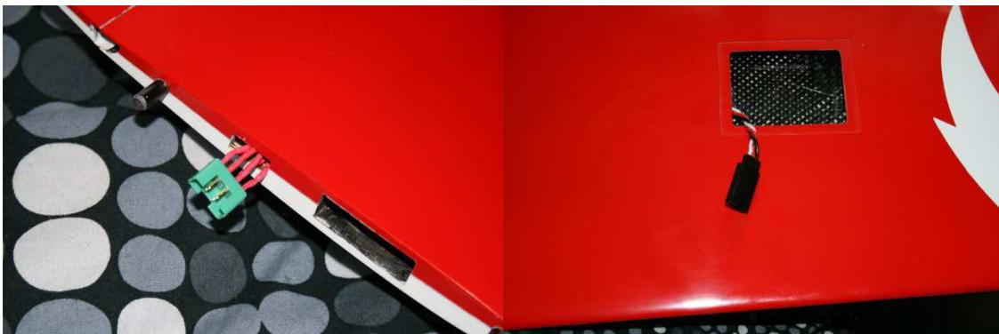
Before installing the servos, put in neutral for the aileron servos. Provide an offset of 20 ° for the flap servos. This is to be a large movement of the flaps.
