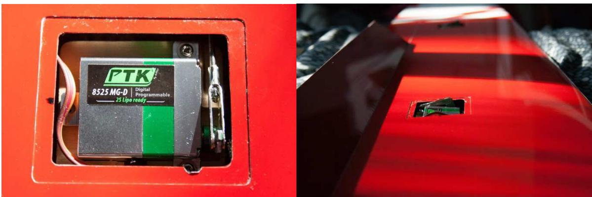
To lock the rod or the operating clearance is too high, you can add a drop of cyano on the spreader and the horn.
