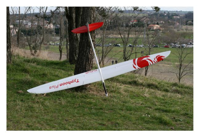
TYPHOON Plus is the big brother of the typhoon 2m. with a wingspan of 2m90, it's a f3f glider. The quality of construction allows it to fly ballast and go fast without any problem. You have as much fun to fly this version of the typhoon thanks to its maneuverability and kindness in flight.
