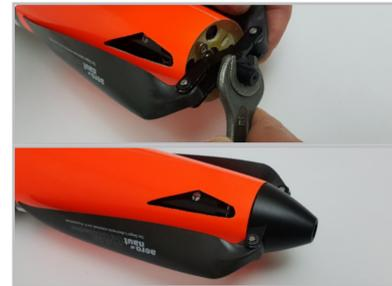
Mount the airscrew center section with propeller blades on the motor shaft. Pay attention to a firm but sensitive tightening of the nut. This is an aluminum thread!
