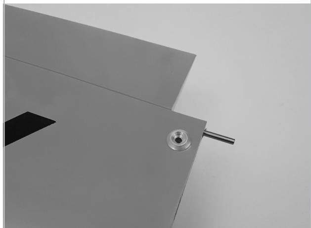
Use epoxy to glue the aluminum pressing disk into the drill holes on the upper side of the wing. Remove the plastic sheet beforehand. Then use the wing screws to fix the wing. Glue the 3mm torsional pin into the root rib of the right part of the wing (slightly roughen and degrease the adherend at first).
