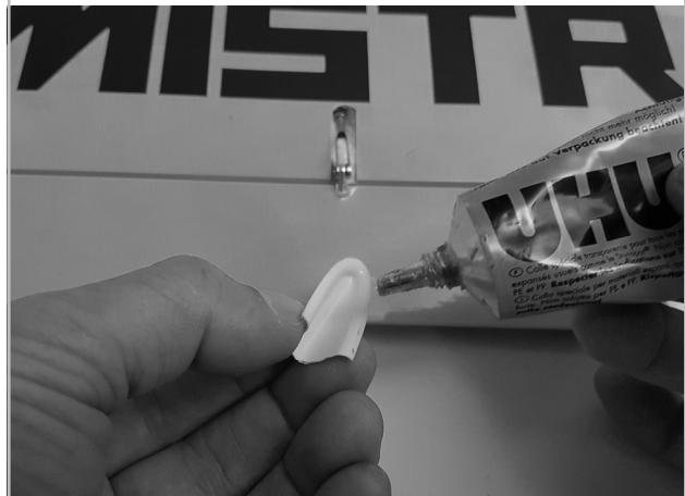
After all electrical adjustments are finished and the rods are finely adjusted; use UHU-Por to glue the servo opening covers and rod covers.
