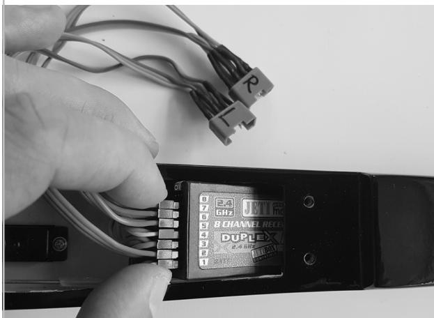
Use velcro tape on the bottom of the fuselage or fixing foam to fix the receiver and all wire leads behind the wing screws.
