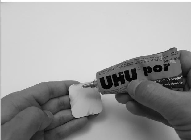
Use the cover to seal the servoshift. In order to glue the cover to the frame of the shaft use UHU Por or double-sided tape.
