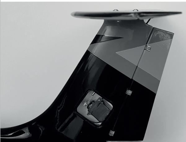
Check the length of the elevator linkage and, if needed, adjust it by adjusting the length of the clevis rods. The rudder should be placed in neutral position during a 90°position of the servohorn.
