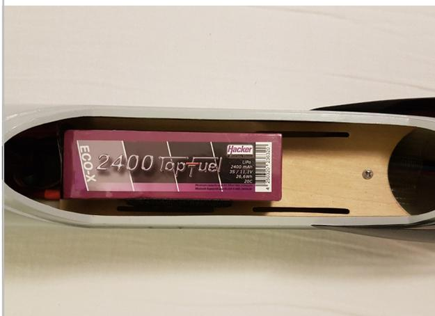
The battery will be fixed by velcro loops on the front battery tray.
