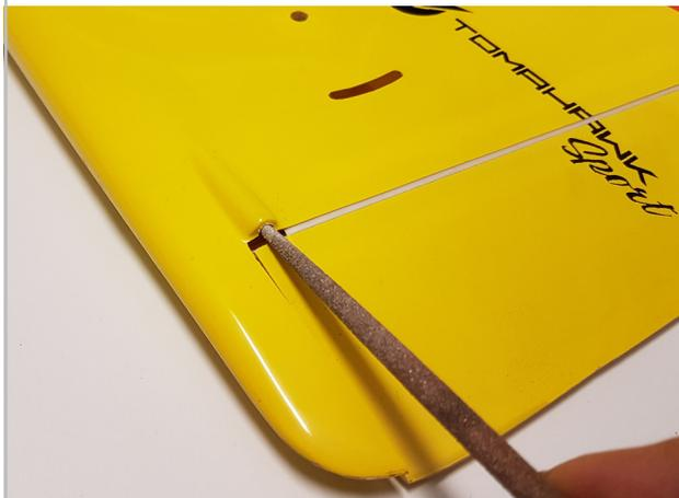
Open the linkage outlet with a small round file.
