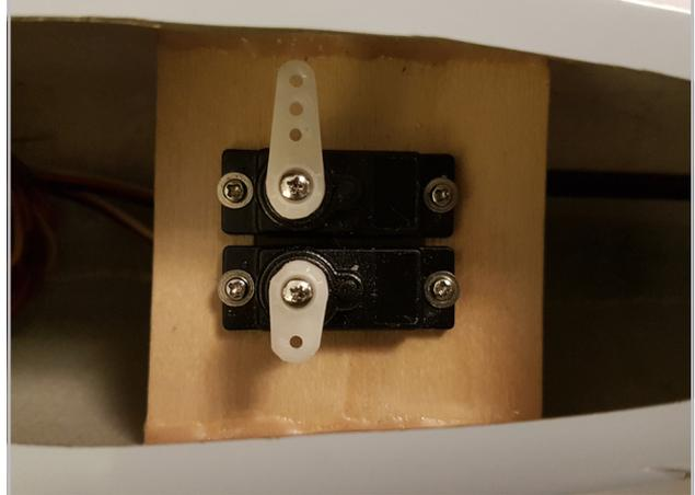
The servos must be placed into the designated wooden frame by already put in neutral position. The servo arm has to be fixed in 90° position.
