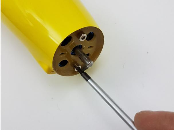
First install the motor on the motor mount by two Allen screws. Then attach the spinner to the motor shaft and the propeller blades.
