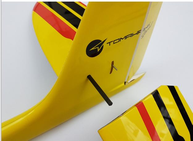
The elevator is connected to the fuselage by the carbon tube and the 2mm steel wire through the bore of the pivot arm.
