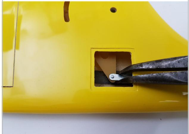
The elevator linkage will be installed and adjusted also at 90° servo position.
