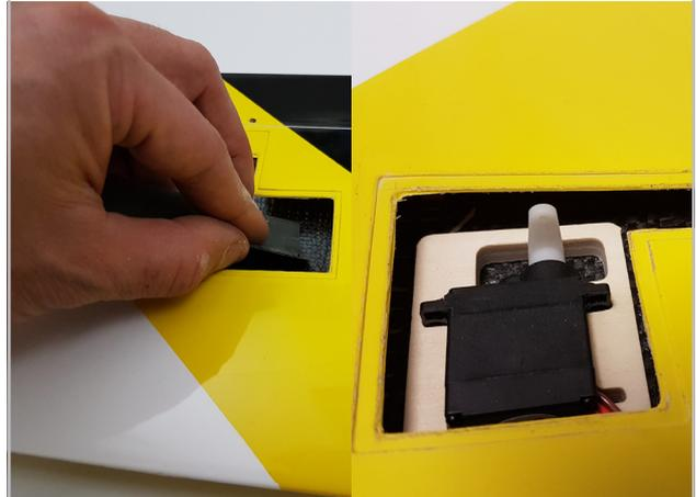
ARF: Install the servo in the servo opening. We recommend the use of a designated servo frame. Use a wire to route the servocable through the servo openings. The green 6-pole MPX plugsystem is used to connect the fuselage.
